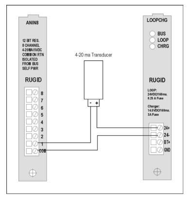
Figure 44 Transducer Hookup (4-20 ma) to 12 Bit Analog Input Board
