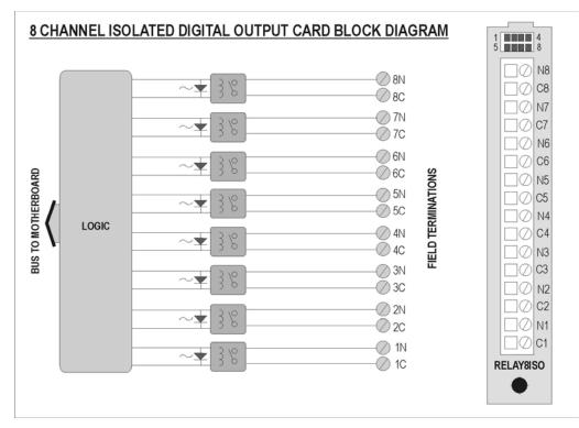
Figure 42 Fully Isolated Relay Output Board Block Diagram
