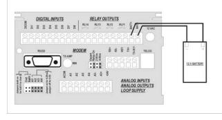
Figure 4 Powering the RUG5 from 12 VDC
