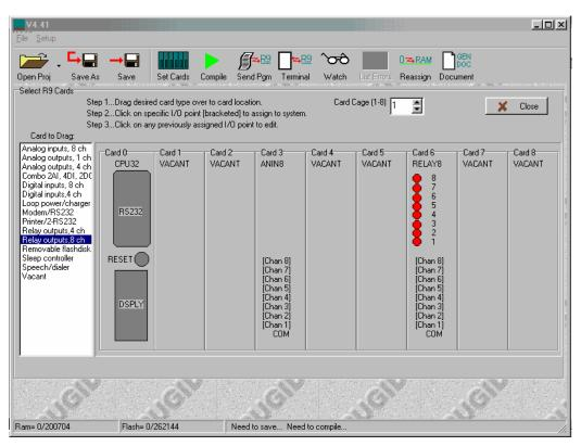
Figure 5 Card Cage with AI and Relay Cards Installed
