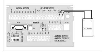
Figure 4 Powering the RUG5 from 12 VDC
