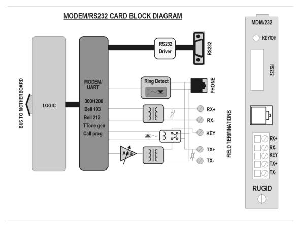
Figure 50 Modem Board Block Diagram
