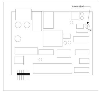
Figure 54 Dialer Board Volume Adjustment Potentiometer Location
