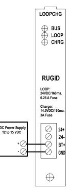
Figure 2 Powering the RUG9 from 12 VDC
