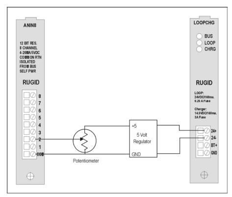
Figure 45 Potentiometer Hookup (0-5Vdc) to 12 Bit Analog Input Board
