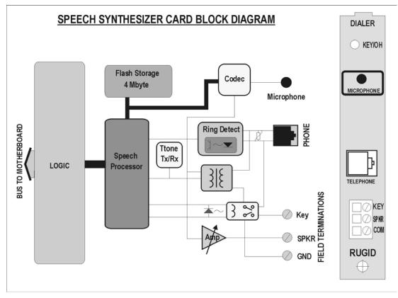
Figure 55 Dialer Board Block Diagram
