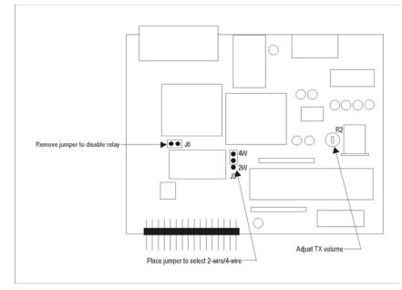
Figure 51 Modem Board User Alterable Features
