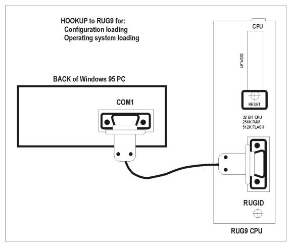
Figure 3 Serial Port Hookup to RUG5/9 CPU
