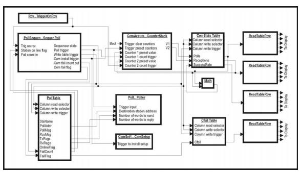
Figure 135 Communications Control and Statistics Block Diagram
