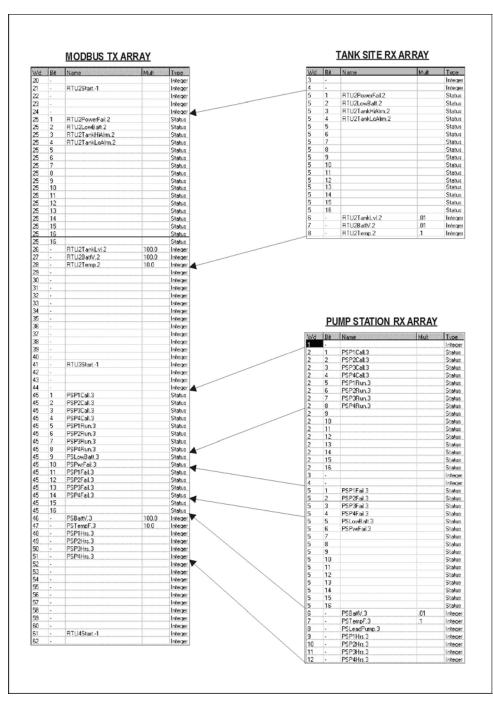
Figure 134 Dragging Data from RTU RX Arrays to Modbus Array
