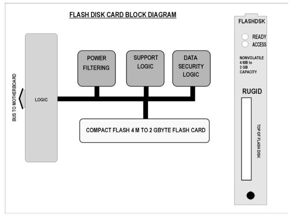
Figure 58 Flash Disk Board Block Diagram
