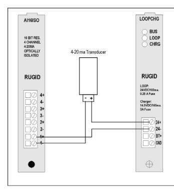
Figure 47 Transducer Hookup (4-20 ma) to High Resolution Analog Input Board
