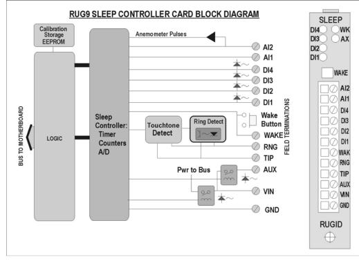
Figure 56 Sleep Board Block Diagram
