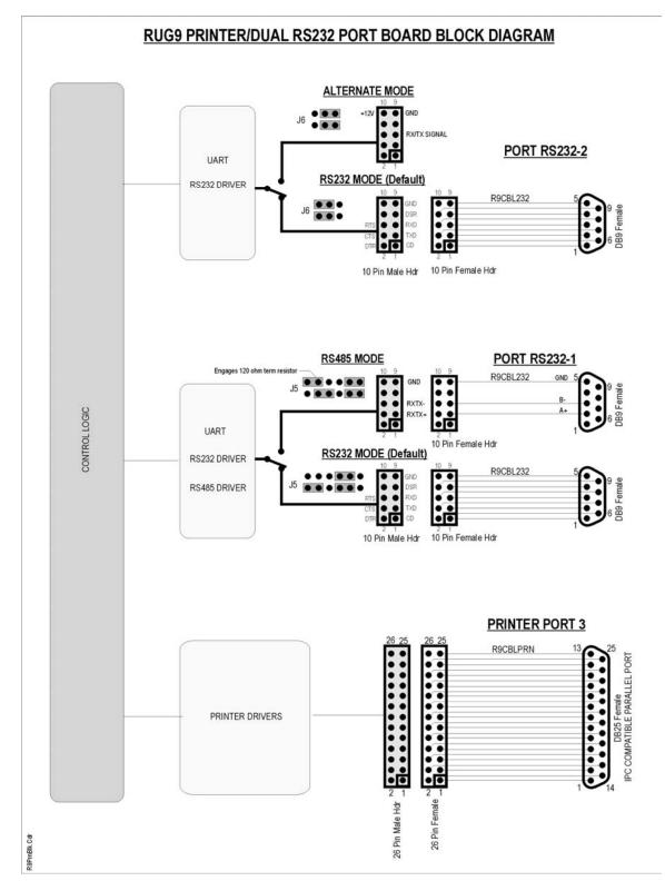
Figure 61 Dual Serial Port/Printer Port Board Block Diagram
