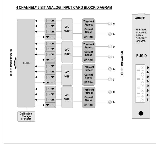
Figure 46 High Resolution Analog Input Board Block Diagram
