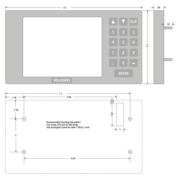
**Figure 146 Display Module Dimensions**
