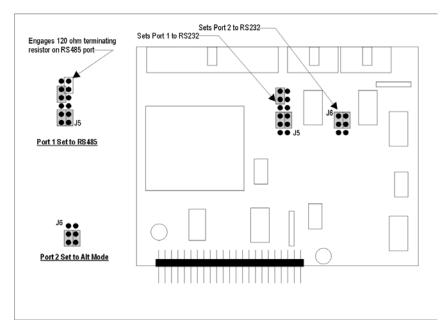
Figure 62 Dual Serial Port Jumper Location
