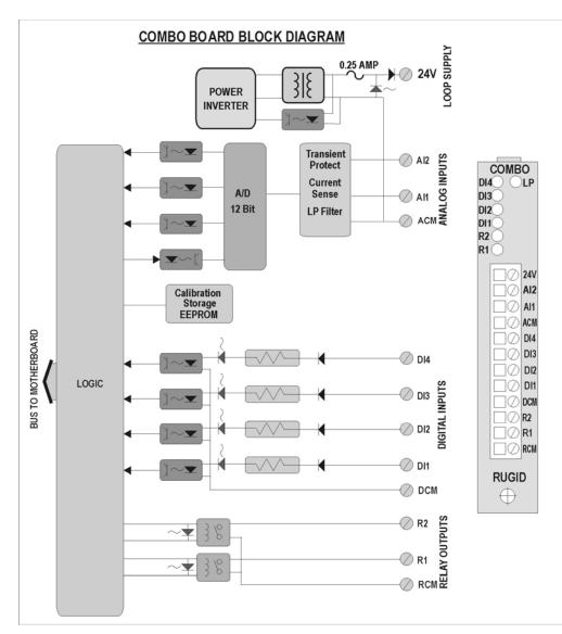
Figure 59 Combo Board Block Diagram
