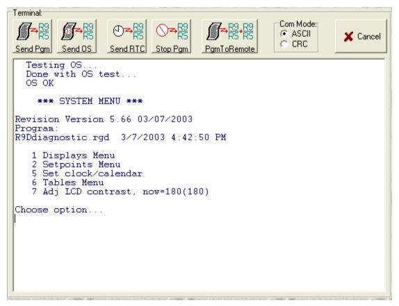
Figure 76 Terminal Page Showing Normal RUG5/9 Boot Up Messages
