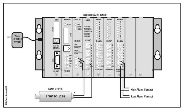
Figure 115 Tank Level Monitor Application
