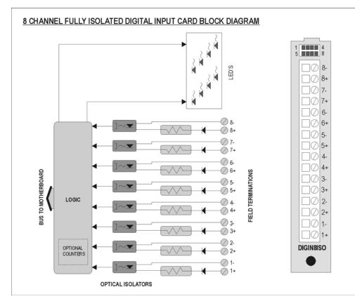
Figure 40 Fully Isolated Digital Input Board Block Diagram
