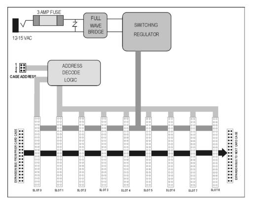
Figure 28 RUG9 Mother Board Block Diagram
