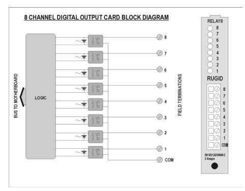
Figure 41 Relay Output Board Block Diagram
