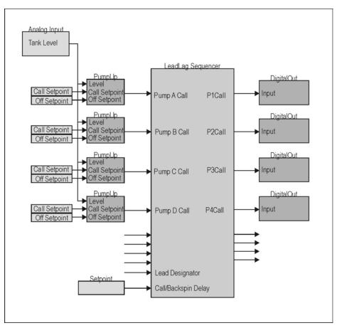
Figure 120 Four Pump Control Logic Diagram
