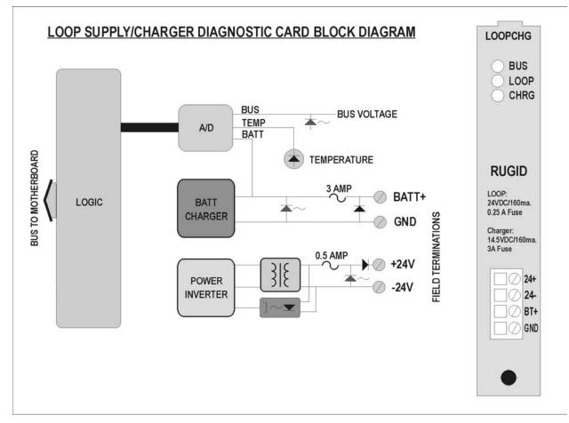
Figure 37 Loop Supply/Charger Block Diagram
