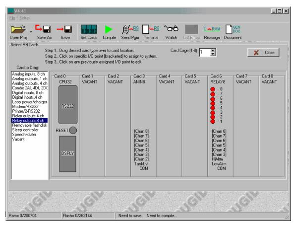
Figure 8 Card Cage With I/O Modules Installed
