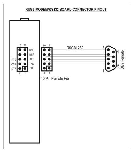
Figure 52 Modem Board RS232 Connections
