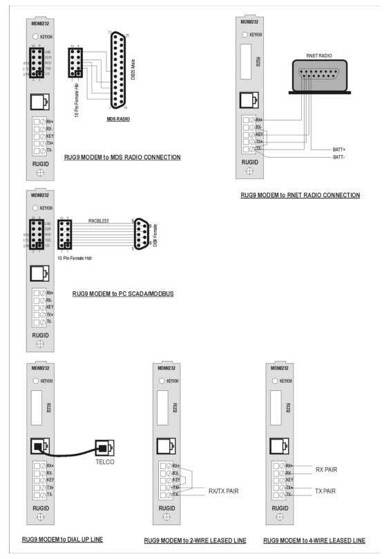
Figure 53 RUG5/9 Modem Typical Connection Examples
