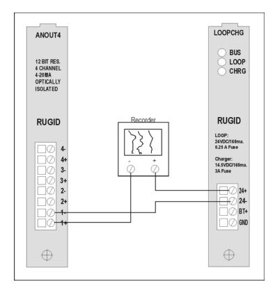
Figure 49 Typical Analog Output Hookup
